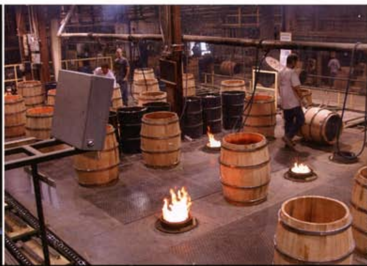
Assuring the quality and repeatability of unique toasting profiles, a cooper (left) at Missouri Cooperage in Lebanon Mo., monitors the toasting process by time and temperature.
