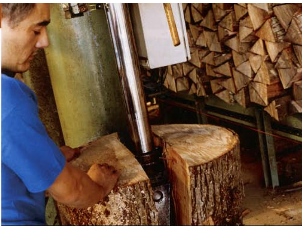
A cooper splits French oak at Taransaud mill in Segonzac, France. Hungarian oak must be split in the same manner.
