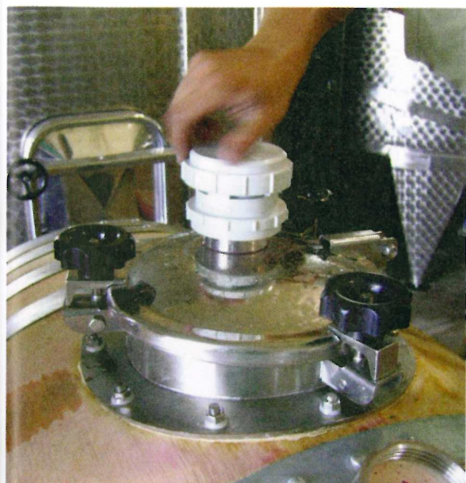
The rotary oak fermentor by Fabbrica Botti Gamba is equipped with a fermentation lid.
